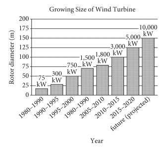
Power rating for each rotor diameter is indicated above the bar.
